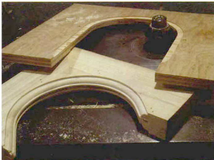
4. Curved stops. Curved stops were made by bandsawing their inside radius in a poplar scrap, molding the radiused edge on the shaper (guided by a template), bandsawing the outside radius and smoothing with a disk sander.
